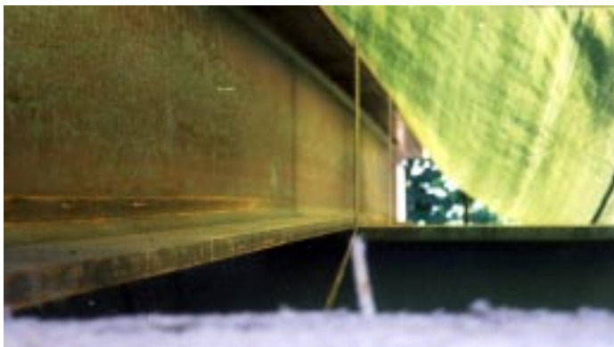
Fig. 84. Deflections in the reaction beams at the end of the loading test on the largest plate.
